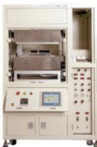
Quartz Chamber Organic compounds, on the silicon wafer placed on the cell, vaporized by heating in the furnace are purged with carrier gas (He) and transferred into the trap unit as sample gas. The possible size of measurement is from 3 to 12 inches (300mm).
