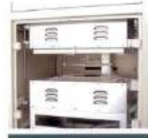
Furnace A Silicon wafer placed on the quartz cell is heated here and organic compounds are desorbed. Operating temperature range is between 100°C to 700°C.
