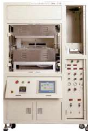
Quartz Chamber Organic compounds, in the silicon wafer placed on the cell, vaporized by heating in the furnace are purged with carrier gas (He) and transferred into the trap unit as sample gas. The possible size of measurement is from 5 to 10 inches (100mm).
