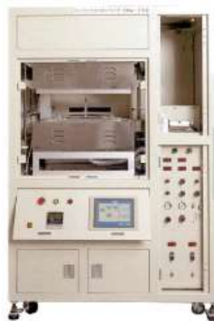
Quartz Chamber Organic compounds, on the silicon wafer placed on the cell, vaporized by heating in the furnace are purged with carrier gas (He) and transformed into the trap unit as sample gas. The possible size of measurement is from 3 to 12 inches (300mm).
